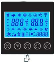
Press the button  $\bigcirc$  to enter the clock setting interface. Clock display on right bottom flashes. Change the hours using and and to go to minute setting, change the minutes using the and and Press again to confirm the setting and return to the main menu. 6.7 Timer setting Hold the button () for 3 seconds to enter the setting of Timer ON & Timer Off groups.
