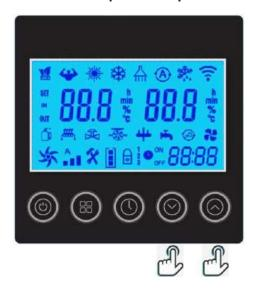
On the main interface, press and to adjust the desired water temp. of your pool, then press the to save the setting.
